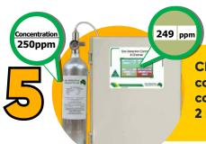
Check the gas concentration on the controller screen after 2 minutes
